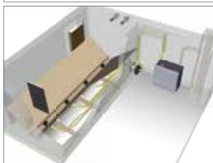
A 30-kg day bin in the boiler reduces the duration of pellet transport to 1 or 2 5-minute feeds per day, and you can set the preferred time of day for transport in the control system.
